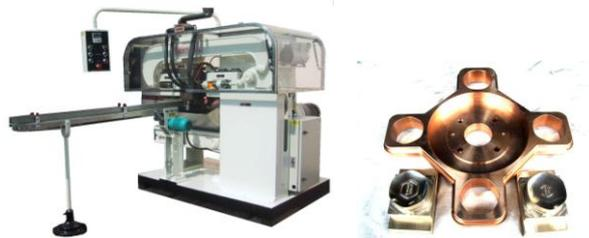
REVOLVER type stamping machine and its banded dieset
