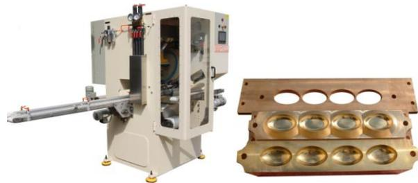
Vertical type stamping machine and its bandless dieset
